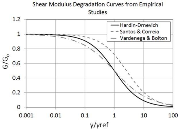
Fig. 2. Reduction curves from fitted experimental data studies
