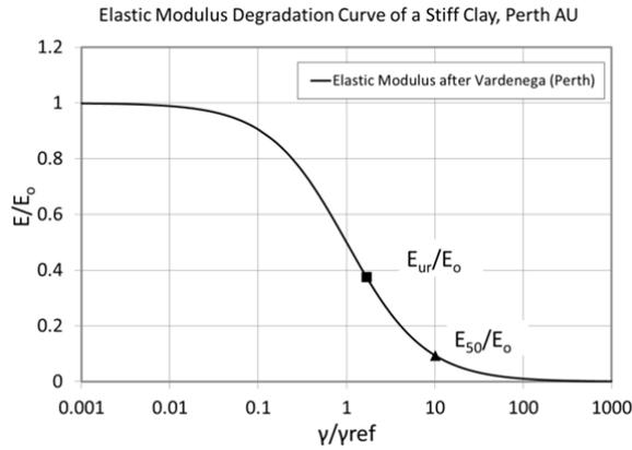
Fig. 7. E- $\gamma$  modulus degradation curve
